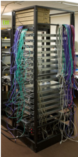
DNS performance testbed rack seen from left rear corner. The cardboard boxes at the top hold racking supplies.
