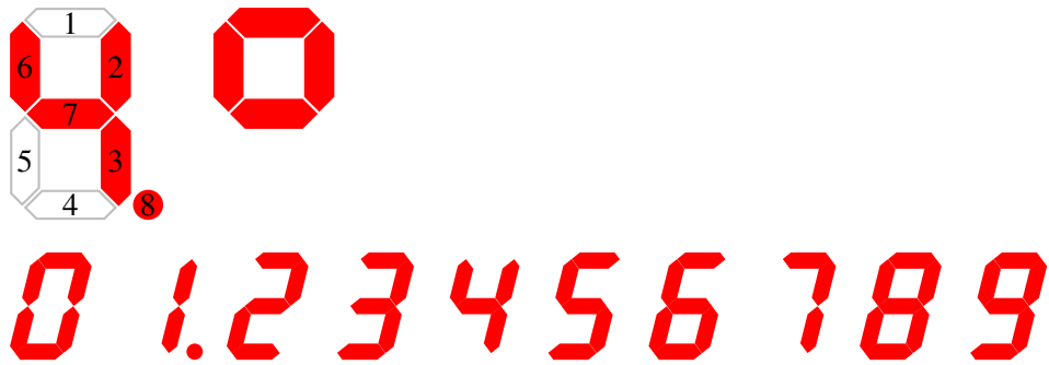
Figure 88: A customizable seven-segment display showing the numbered segments, a custom shape, and the numerals from 0 to 9 [Sevensegment.m4].
